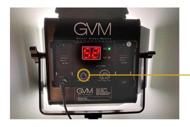
Set the LED light panel's color temperature by rotating the left dial on the rear control section of the light. Set the intensity (10-100%) with the right dial.
